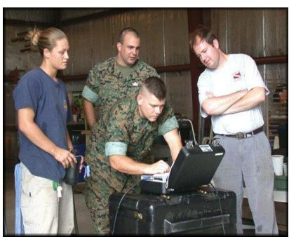
X-raying at the QAR Lab In July's report we mentioned concretion **QAR495.000**, and our desire to have it x-rayed. The size, weight and fragility of this concretion makes travel difficult, so on September 9th, Sqt. Foster and SSqt. Leonard, of the Explosive Ordinance Disposal (EOD) at the Marine Corp Air Station in Cherry Point, helped us out once again by coming to the QAR lab. Their portable x-ray unit was set up in our warehouse where OAR495.000 and a few other objects were x-rayed.
