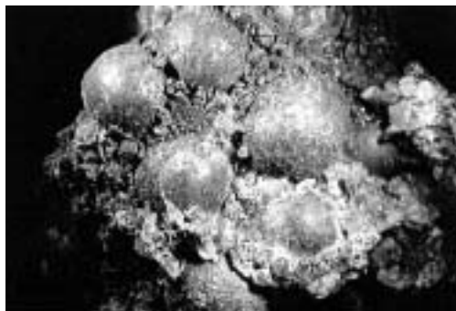
Figure 2. Cemented mass of lead shot and interstitial sand. This material has been extracted as solid masses which are cemented by a mixture of lead oxides, hydroxides, and sulfide (See also Figure 5).
